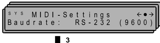
■ 3, Baudrate: MIDI (31250)   RS-232 (9600). Use RS-232 and the supplied cable to remote control the device with the help of a PC via one of it's serial-interfaces (COM#) or to re-load presets or to update the operating system. Use MIDI, to link several DSC28-controllers by means of a standard MIDI-cable (📖 Chap.19).
