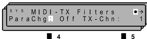
■ **4, ParaChg: Off** **On** . If this value is set on On, the device sends all performed parameter-adjustments out. As such several device (Slaves) can be commonly operated by one device (Master).
