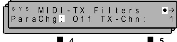
■ 4, ParaChg: **Off** **On**. If this value is set on On, the device sends all performed parameter-adjustments out. As such several device (Slaves) can be commonly operated by one device (Master).
