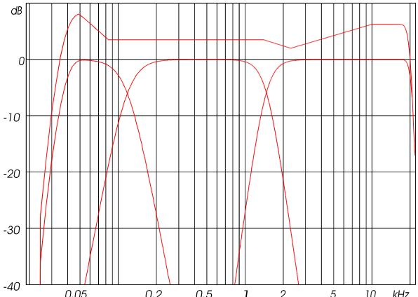
**Figure 14.2** Target-functions, system (weighted) and band-passes
