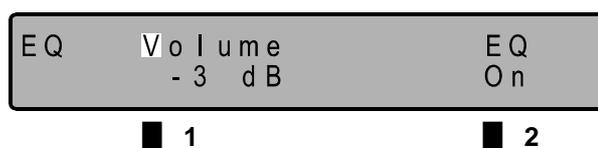
■ 1, Gain: -24dB ↻ O -3dB O 0dB, 1dB steps. Should the activated EQ-bands be solely used for frequency reduction then a value of 0dB is recommended. Should however, frequency-boosts also be applied then a gain-reduction in accordance with the highest boost-value is recommended.
