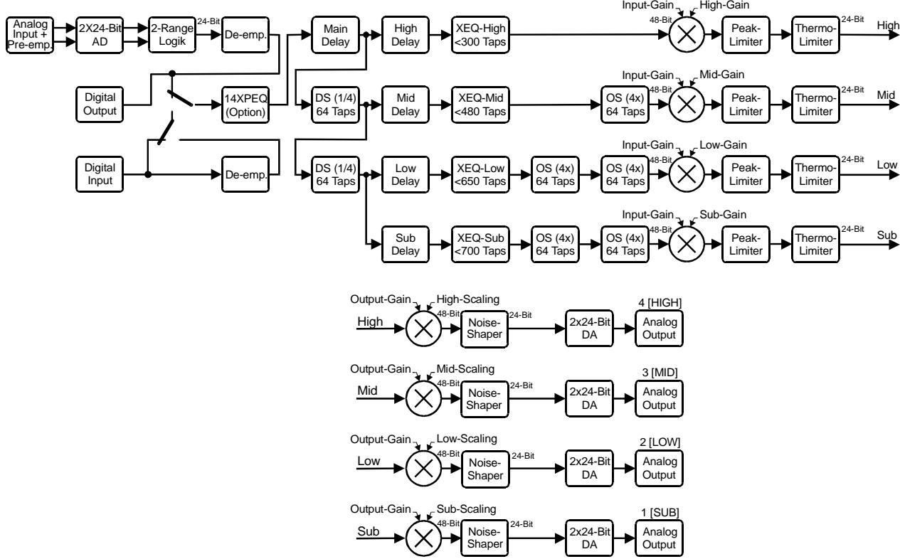
**Analog input.** After passing through an analog pre-emphasis filter, the analog input leads to two different amplifier stages with different gain-rates, which drive both inputs of the 24-Bit Stereo AD-converter.
