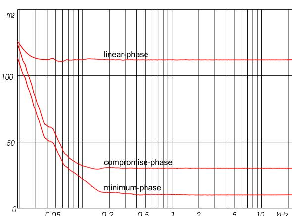
**Figure 14.7** Equalised system, 3 examples of total delay response
