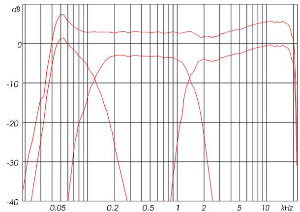
**Figure 14.6** Equalised system, total frequency response, single frequency responses
