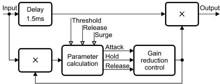
Figure 15.2 Pre-viewing digital peak-limiter
