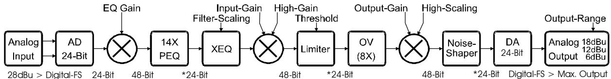
**Fig. 12.1 Gain architecture.** Fig.6.1 is an extract of the block-diagram and shows the signal-flow using the example of the HIGH-path. Only modules wholly or partly relevant to gain are considered. (The \* at \*24 bit indicates: reduction from 48-bit to 24 bit by means of a noise-shaper with 1<sup>st</sup> Order-Error-Feedback).
