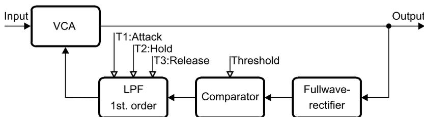
Fig. 15.1 Analog peak-limiter
