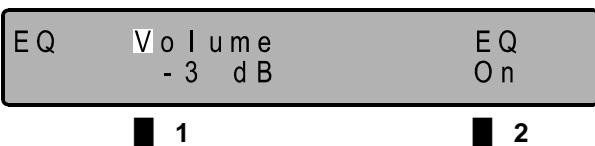
■ 1, Gain: -24dB ↴ O -3dB O ↵ 0dB, **1dB steps**. Should the activated EQ-bands be solely used for frequency reduction then a value of 0dB is recommended. Should however, frequency-boots also be applied then a gain-reduction in accordance with the highest boost-value is recommended.
