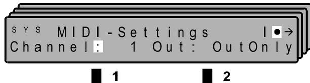
■ 1, Channel: 1   16. Assign the controller-address (basic channels 1-16), at which data can sent and received.
