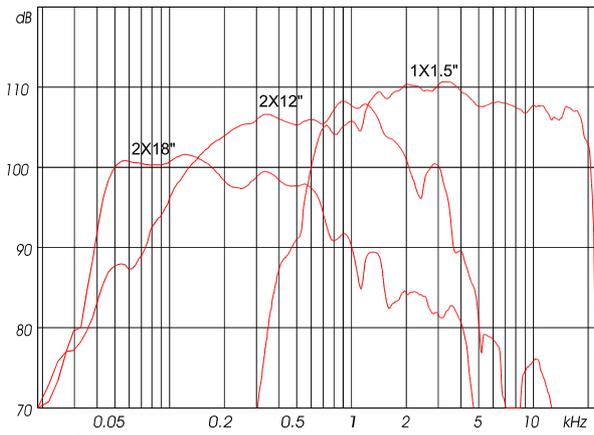
**Figure 14.1** Loudspeaker-system, single measurements of the components, sensitivity @ 1W, 1m
