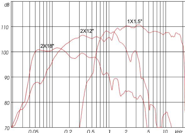
**Figure 14.1** Loudspeaker-system, single measurements of the components, sensitivity @ 1W, 1m
