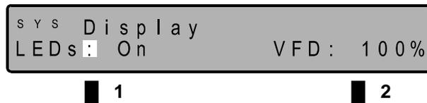
■ 1, LEDs: Off   On. Here the LED-display can be turned on or off. The status LEDs remain on.
