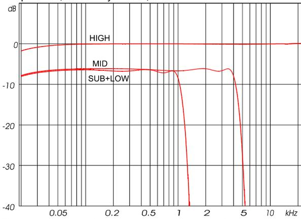
**Figure 14.3** Controller-intrinsic-response, amplitude
