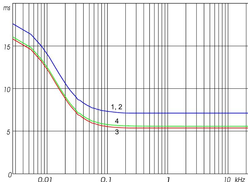
**Fig. 13.3 Intrinsic run-time behaviour.** The basic run-time of the four paths is represented by the values of the linear-phase segment of the delays, including the delay of the "pre-viewing" limiters (1.5ms): SUB + LOW: 7.2ms, MID: 5.4ms, HIGH: 5.6ms. The minimum-phase segment and the run-time increase towards lower frequencies and are caused by the 1<sup>st</sup> order high-pass filter within the analog-input module (Coupling-capacitor).
